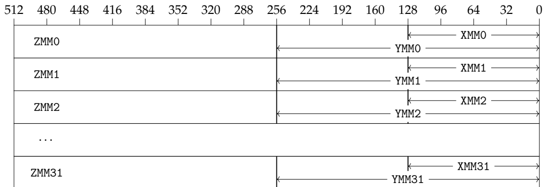
Figure 2.5: Vector registers introduced by SIMD extensions
